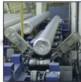
Ultrasonic test of the bars
